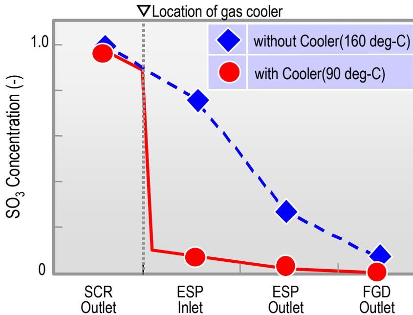
Fig.8 SO<sub>3</sub> concentration profiles in AQCS
