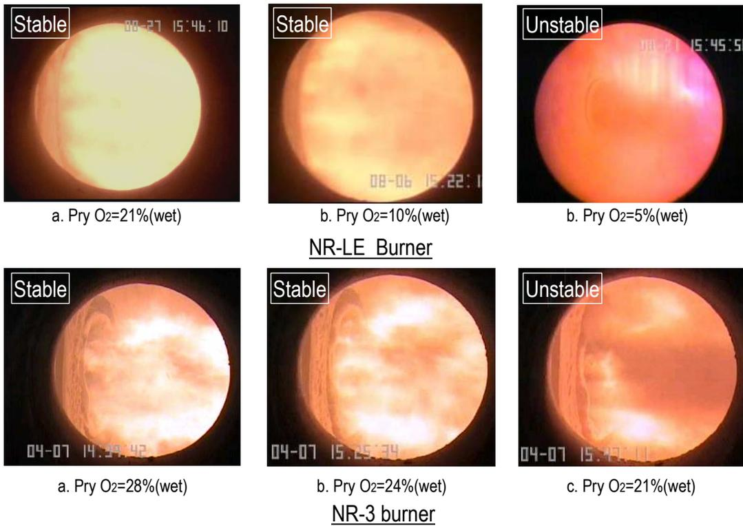
Fig.7 Flame Photographs of Hitachi NR-LE and NR-3 burner (Average O<sub>2</sub> 28%-wet)
