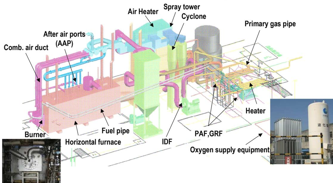
Fig.5 Three-dimensional view of 4MWth combustion test facility
