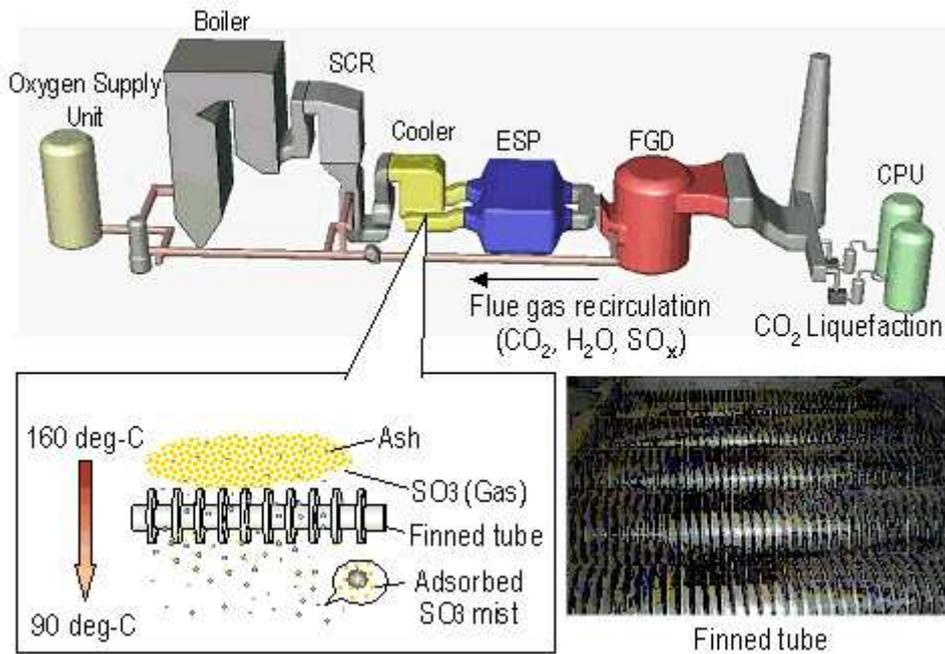
Fig.4 Mechanism of SO<sub>3</sub> removal with cooler system
