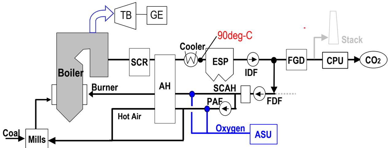
Fig.2 System flow of a Hitachi original oxy-combustion
