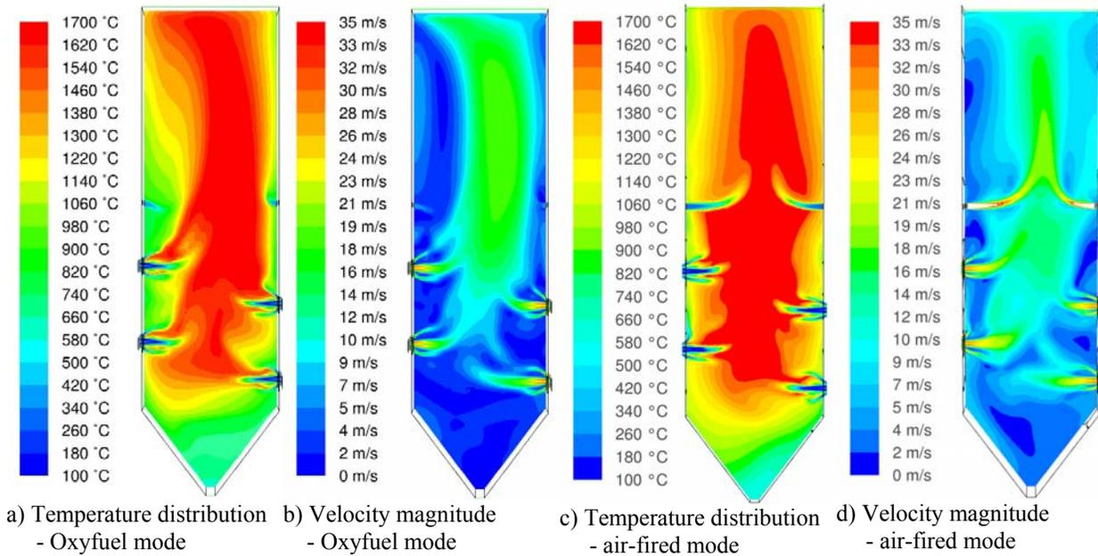
Figure 5: Simulated temperatures and velocity magnitudes in Oxyfuel and air-fired mode
