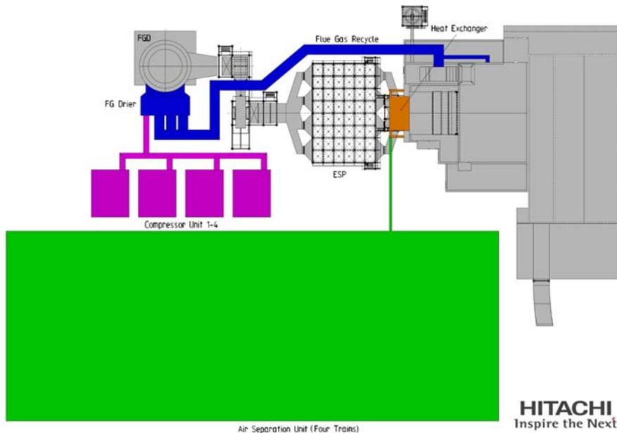
Figure 6: Arrangement for retrofitted power station
