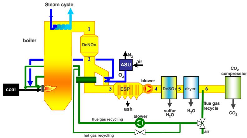
Figure 1: The oxyfuel process
