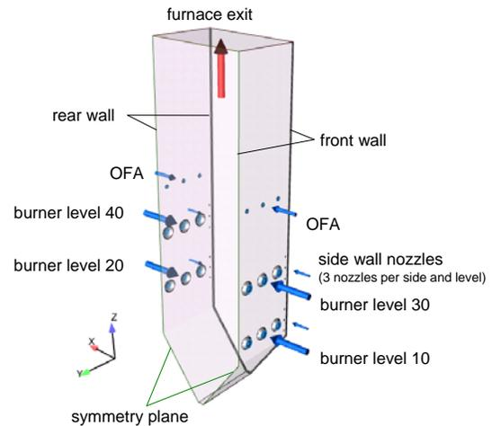
Figure 4: Furnace geometry
