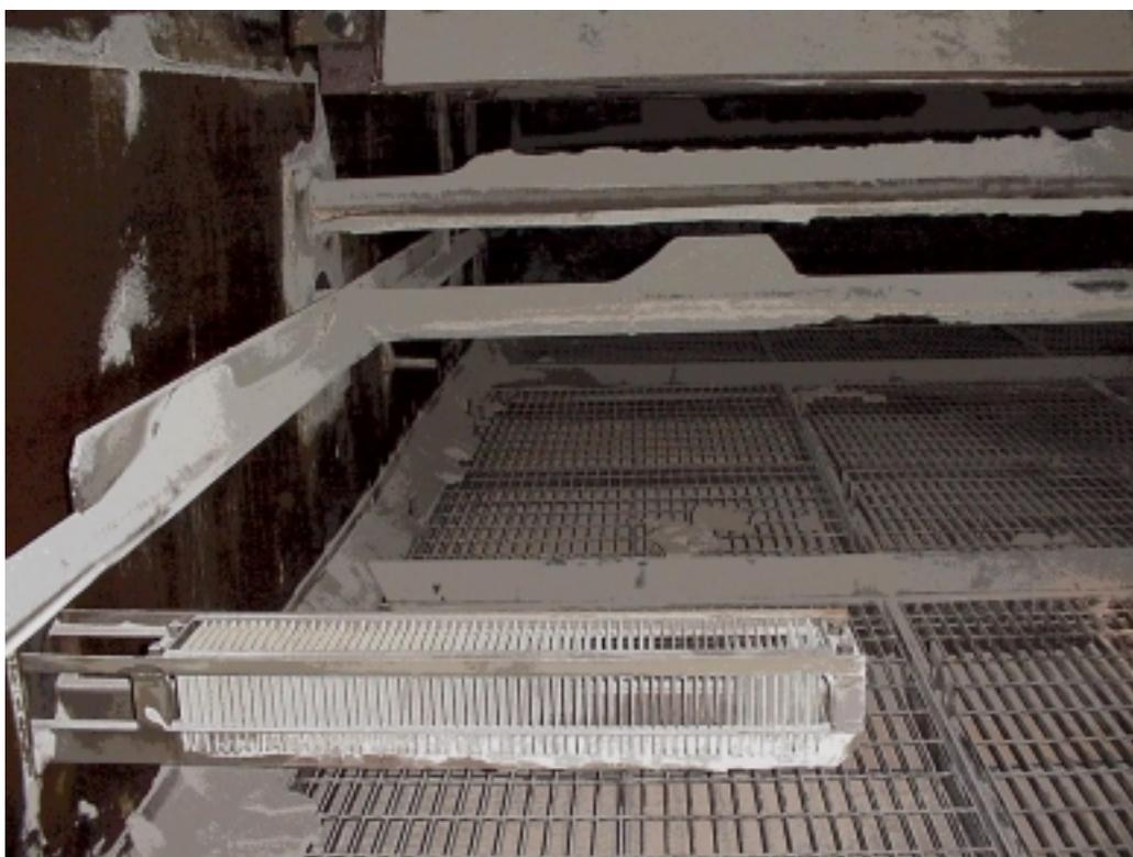
Plate 8: Catalyst Test Coupons in Cassette
