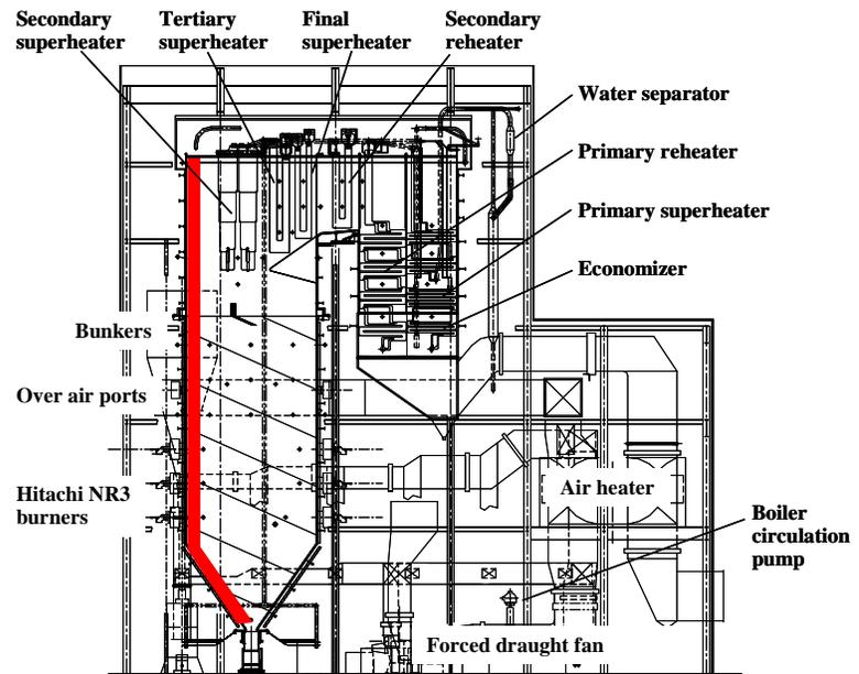
Fig. 4 Side View of Genesee Phase 3 Boiler
