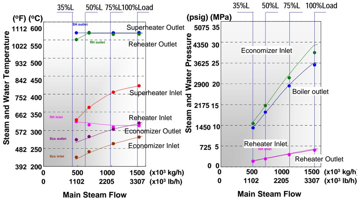
The load change characteristics of the boiler are shown in Figure 13. Due to the well established main steam and reheat steam temperature control, stable temperatures within the allowable tolerance were confirmed with sliding pressure condition.
