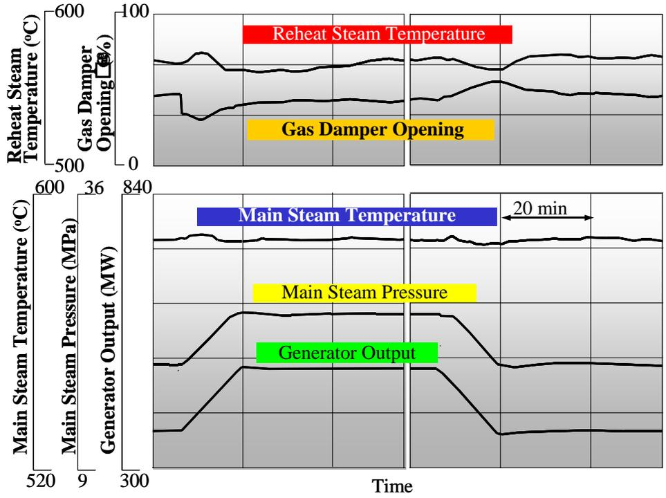
Fig.12 Boiler Characteristics at 100% Load
