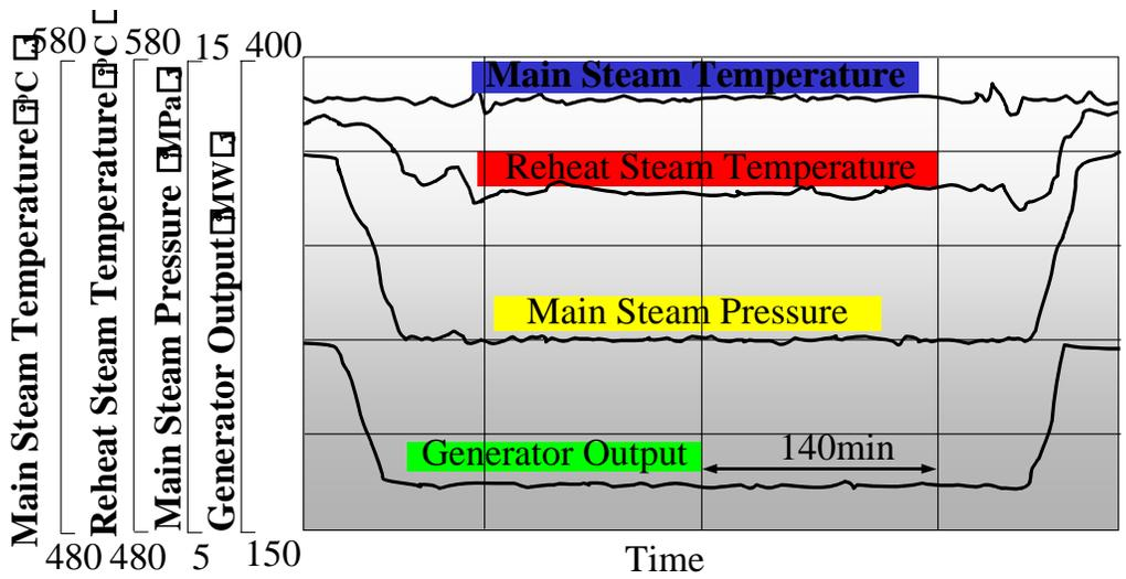
Fig.14 Result of Minimum Load Test at 35% Load
