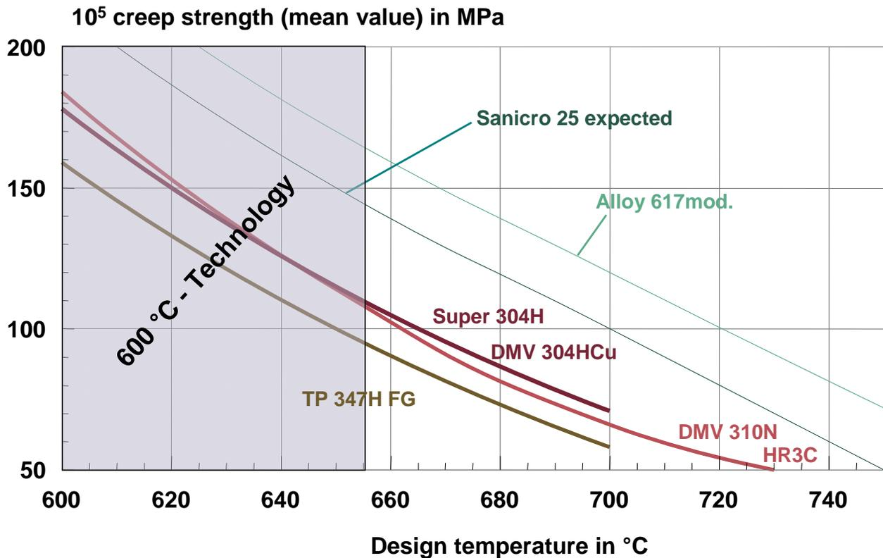
Figure 2-1: Creep strength of austenitic materials and nickel base alloys
