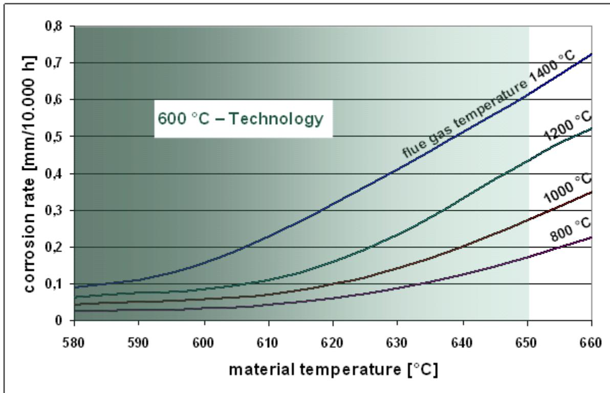
Figure 2-2: Corrosion rate of austenitic materials with 18 % chromium [Source: Cutler, A.J.B., Flatley, T and Hay, K.A.: Fire-side corrosion in power-station boilers. Combustion (Dez. 1980) S. 17-25]
