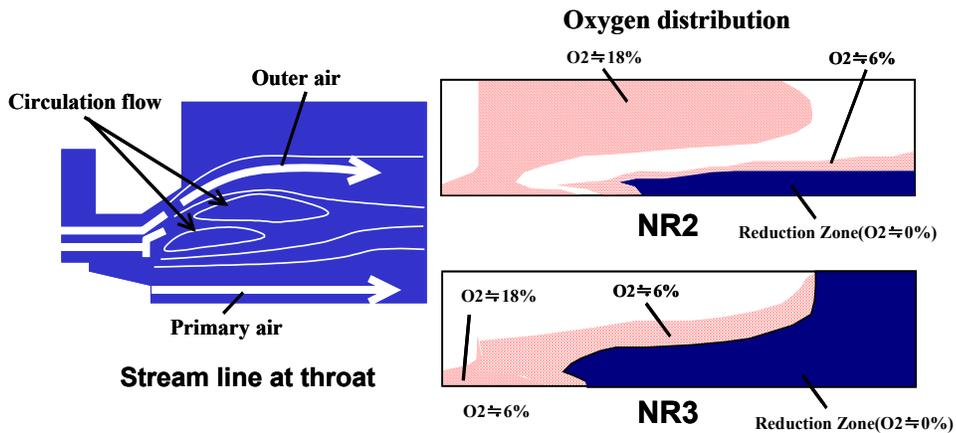
Numerical analysis condition ; Cylindrical coordinates , SIMPLE method ,
