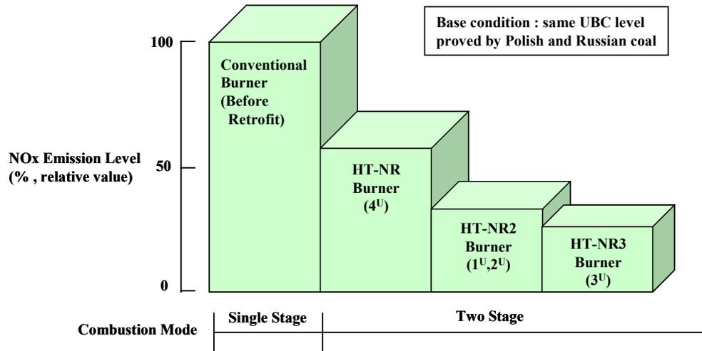
Fig.6 Result of combustion performance test IN
