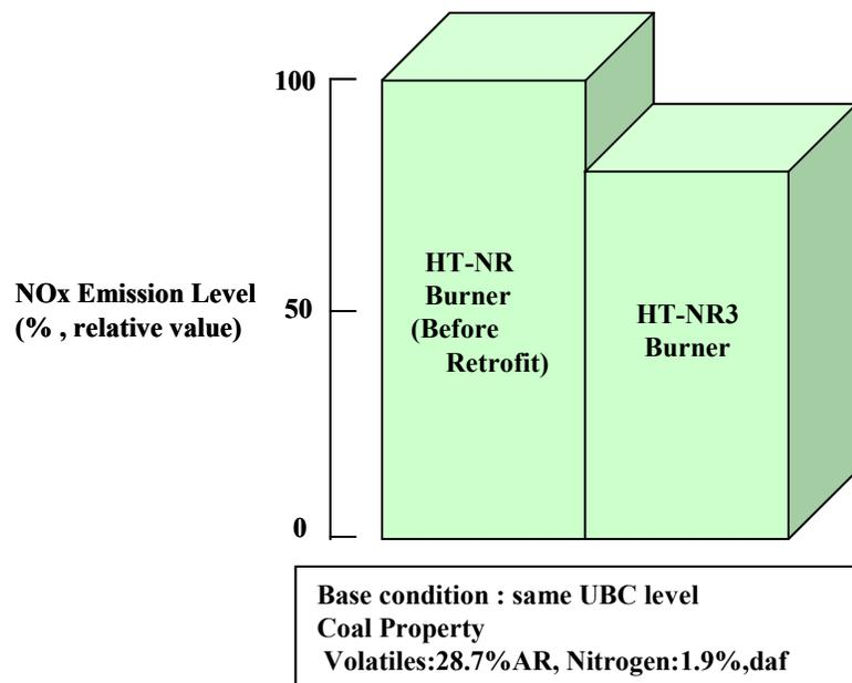
Figure 7 Result of combustion performance test HW
