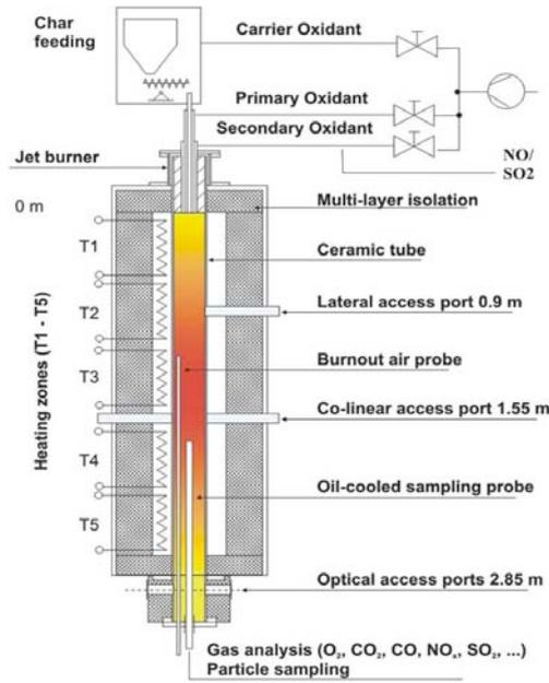
Figure 1. Schematic diagram of the once-through 20 kW furnace [1].
