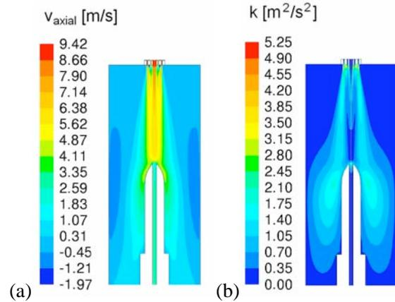
Figure 3. Calculated axial velocities (a) and turbulent kinetic energy (b) for the case of 95 % N<sub>2</sub> and 5 % O<sub>2</sub> and a probe position  $\Delta x = 0.22$  m away from the burner.
