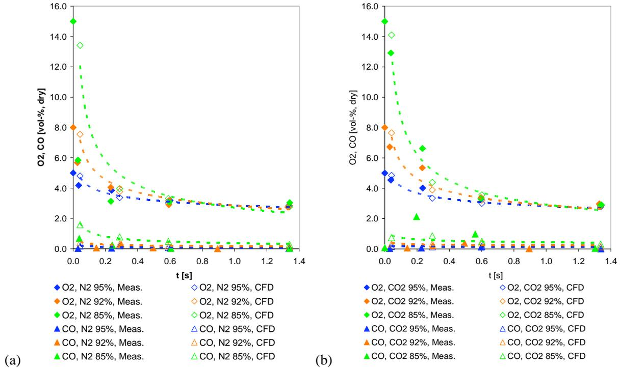
Figure 5. Measured and calculated species volume fractions for six different atmospheres: (a) Values in N<sub>2</sub>-environments; (b) Values in CO<sub>2</sub>-environments. The dashed lines are fit-curves through the values from the CFD-simulations.
