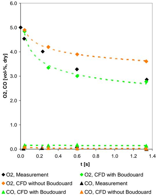
Figure 4. Measured and calculated species volume fractions for the case of 95 % CO<sub>2</sub> and 5 % O<sub>2</sub>. Comparison of CFD-simulations made with and without Boudouard reaction.
