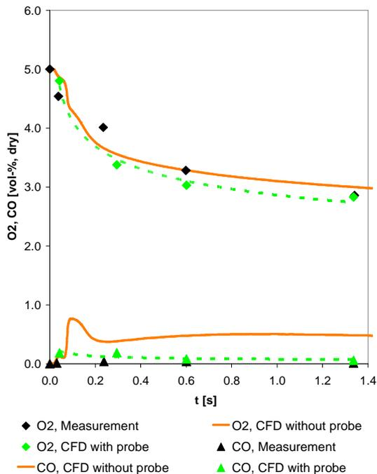
Figure 2. Measured and calculated species volume fractions for the case of 95 % N<sub>2</sub> and 5 % O<sub>2</sub>. Comparison of CFD-simulations made with and without sampling probe.
