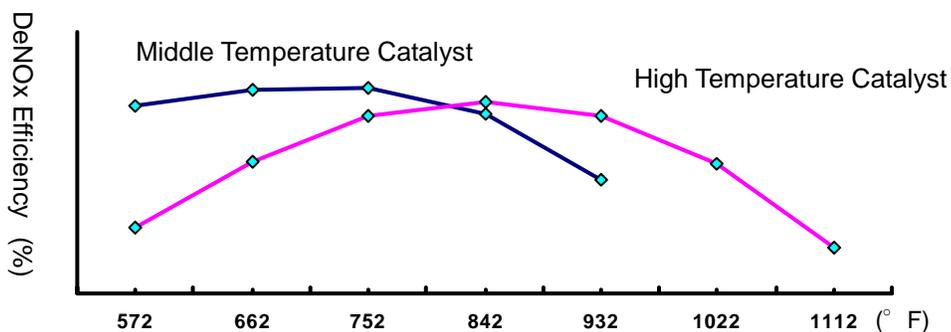
Figure 2 – Efficiency (Activity) with Temperature
