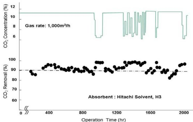
Figure 3: Long-term pilot testing of H3 solvent under various inlet CO<sub>2</sub> concentrations
