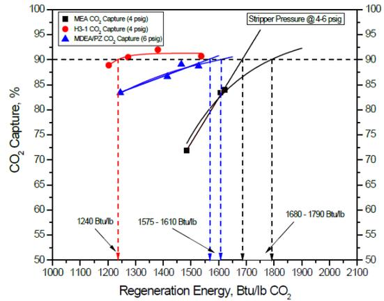
Figure 7: Comparison of Regeneration Energy of Various Solvents
