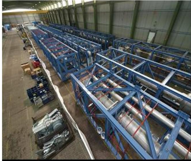
Figure 11. Mobile pilot plant segments
