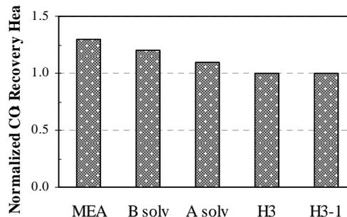
Figure 5: Comparison of CO<sub>2</sub> recovery heat from different solvents
