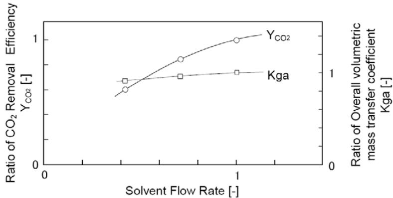
Figure 9: Effect of Solvent Flow Rate on CO<sub>2</sub> Removal Efficiency
