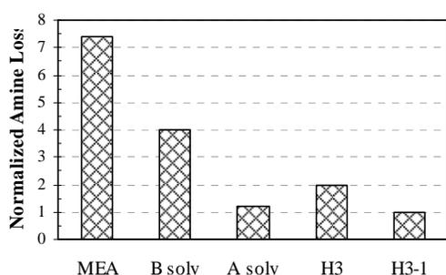
Figure 4: Comparison of Amine Loss from different solvents
