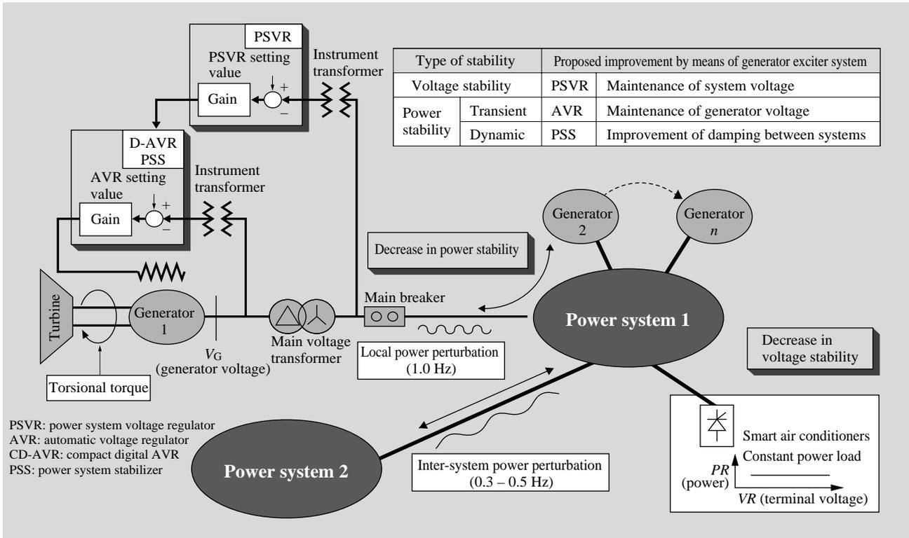
Fig. 1— Power Systems and Stability. Stability includes power stability and voltage stability. Improving both of these is important to the operation of a power system.
