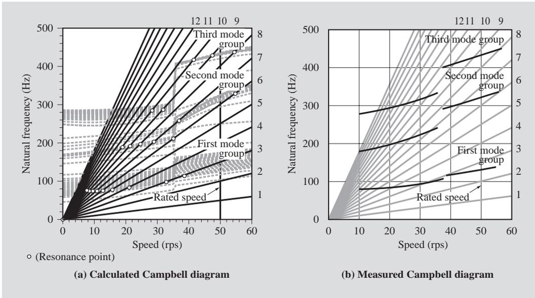
Fig. 8—Comparison of Campbell Diagrams. Both calculated results and measured reliability test results verify excellent vibration characteristics without any resonance points near the rated speed.
