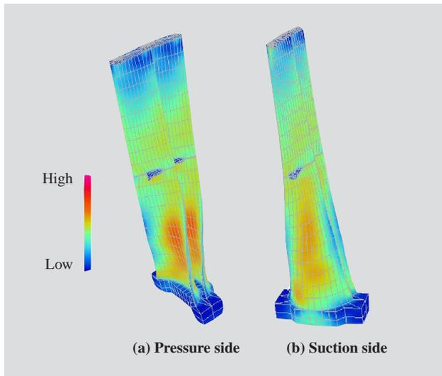
*Fig. 6—CCB Long Blade Analysis Examples (Stress Distribution).
