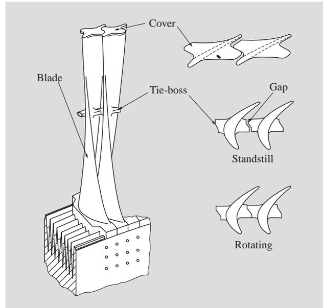
Fig. 5—Schematic Diagram of CCB Structure. Blades are interconnected by shroud covers and tie-bosses. Covers interlock as blades begin to rotate, and tie-bosses interlock once rotation is under way.
