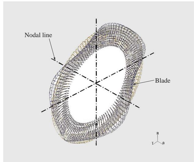
*Fig. 7—Vibration Mode Analysis Example.
