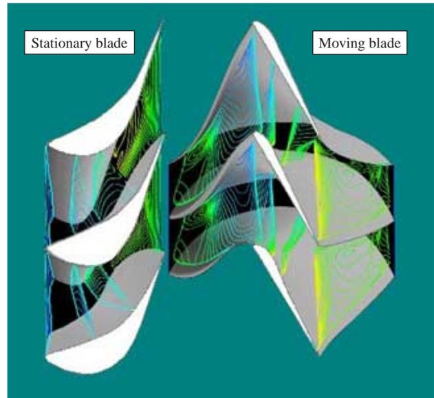
Fig. 2—3D Stage Flow Analysis Example.
