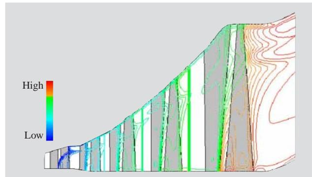
Fig. 3—Wetness Distribution Derived by Nonequilibrium Condensation Flow Analysis.
