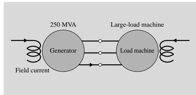
Fig. 4—Rated Field Current Test – Circuit Diagram.
