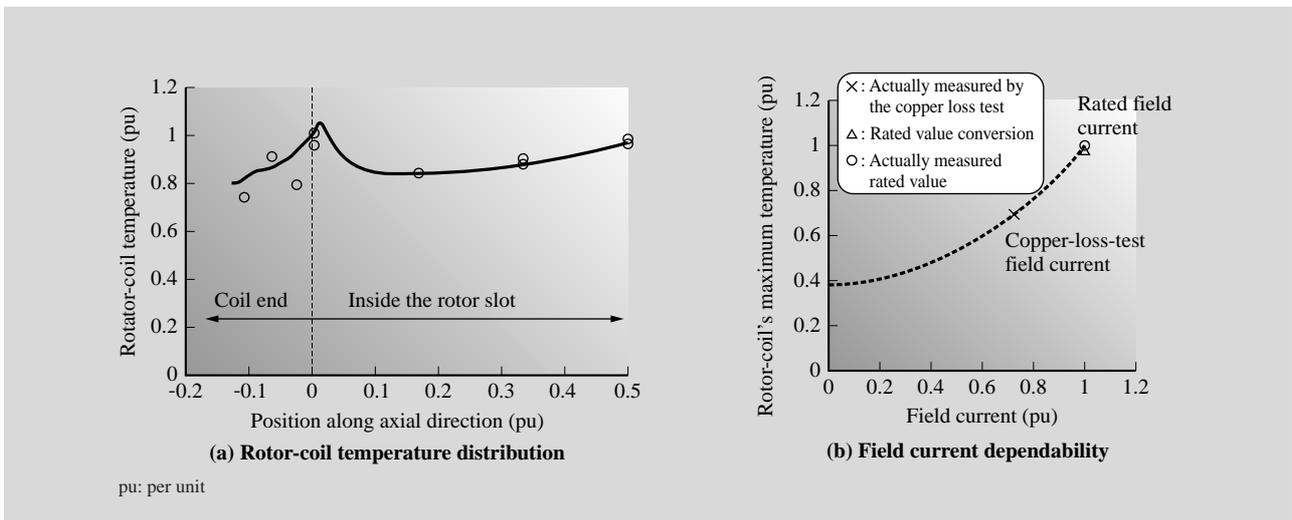
Fig. 6—Rotor-coil Temperature Distribution.
