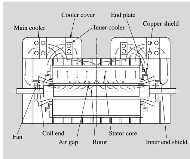
Fig. 2—Schematic of Cooling Method for Inner Cooler Cooling System.
