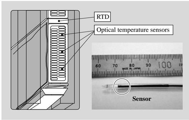
Fig. 6—Schematic of Temperature Measurement by Strand (left) and External View of Temperature Sensors (right). Optical sensors embedded in the stator coil measured the strand temperature.
